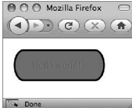
Figure 1-4. A rectangular shape, defined with the <rect> element, is all that's needed to create a background.
