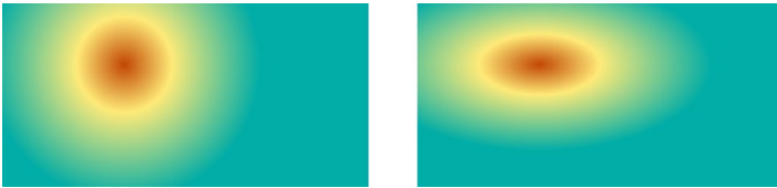
Figure 19-17. The outer edge of each gradient passes through the closest corner of the gradient box
