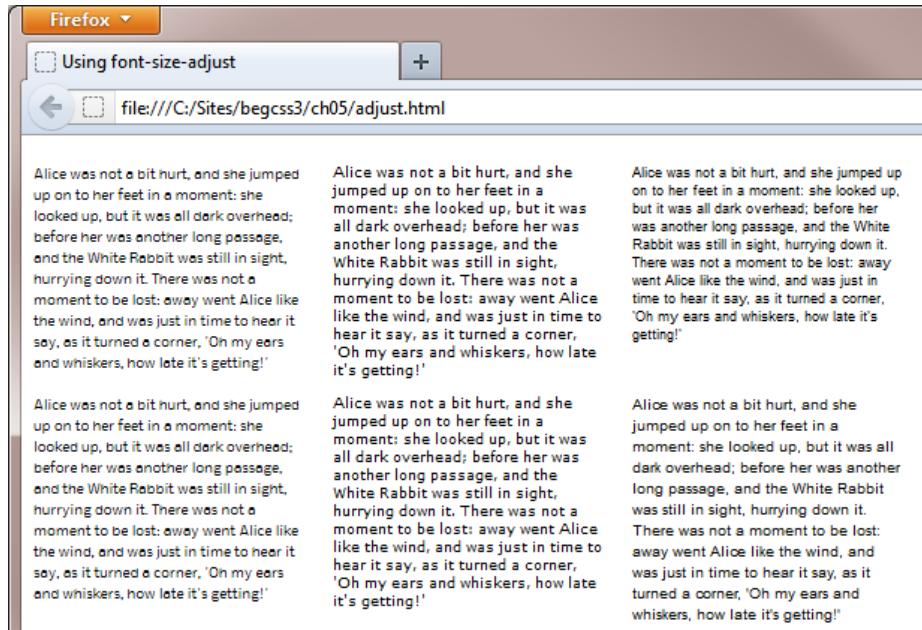
Figure 5-9. Using font-size-adjust changes the size of fallback fonts to match the first choice
