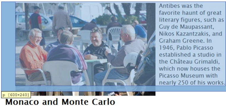
Figure 7-11. The paragraph's margins are not affected by the floating image
