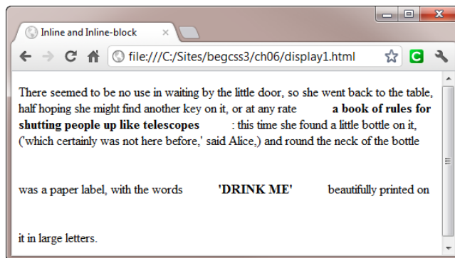
Figure 6-11. Setting display to inline-block affects the line height of the surrounding text
