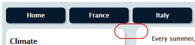
Figure 10-16. There's a slight, but perceptible misalignment with the sidebar in IE 9
