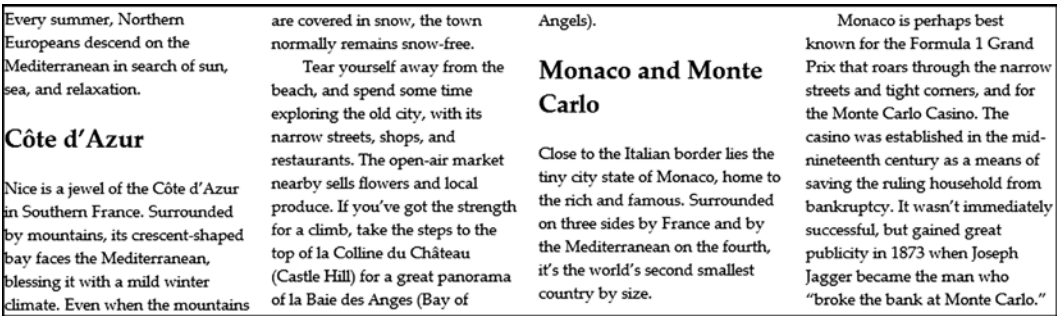
Figure 18-4. The browser adjusts the number of columns to take account of the gap
