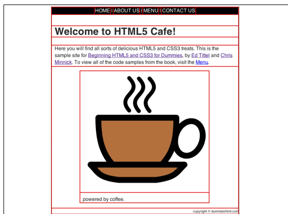
Figure 14-1: CSS draws a rectangular box around each element.
