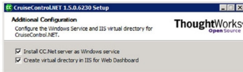
Figure 4.7 You can install CCNet as a Windows service and configure IIS to be ready to serve the Web Dashboard.
