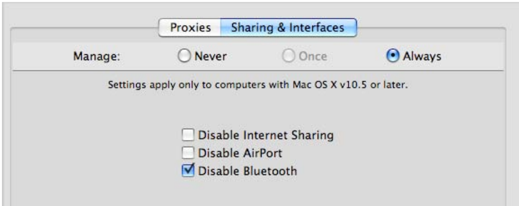
Figure 11-7. Disabling Bluetooth via Network preferences
