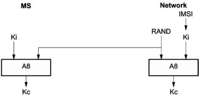
Figure 5.53 Generation of the cipher key K_c .
