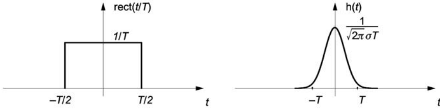
Figure 4.3 Impulse responses for the building blocks of the GSM transmitter filter.
