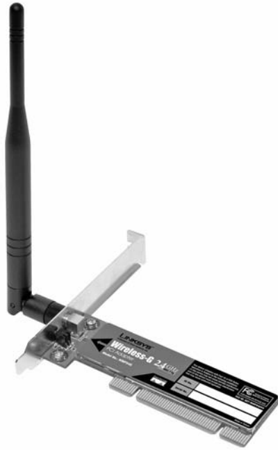
Figure 1-7: A (Wi-Fi) wireless network adapter that goes inside your desktop computer.
