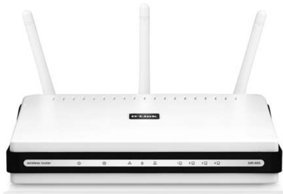
Figure 3-6: A wireless network router, shown here, has at least one antenna; a wired router has none.
