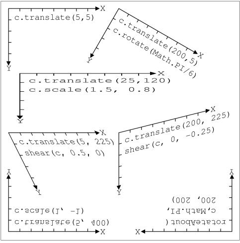
*Figure 21-7. Coordinate system transformations*
