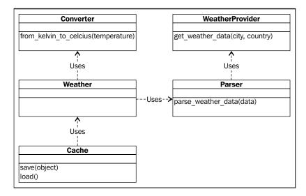
The client will deal with caching, making requests to API, converting, and so on. What if to create a Facade for it? The client will use the get\_forecast method, passing it in two strings: the requested city and country, and the method returns the forecasted temperature for today in Celsius.
