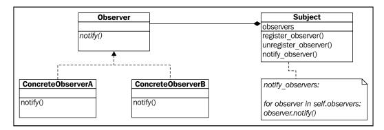
**Subject** is the static part of the system; throughout the application lifetime, there is only one **Subject**. On the contrary, **Observers** are the variable part. There can be many or even zero observers, and this value changes during the lifetime of the application. All the parts that are updated often are typically implemented as **Observers**.
