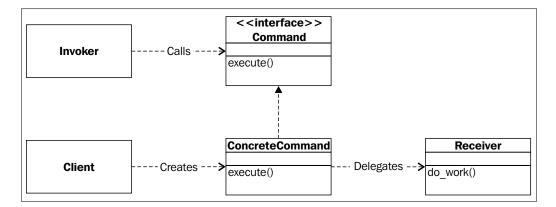
The Command design pattern provides an interface to call a method to perform some job and encapsulates all necessary information to do it in one object call, which can be run separately after instantiation.
