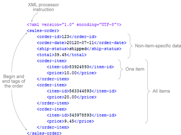
Figure 5.2 A sales order in XML markup format. The file begins with a processor instruction that indicates what version of XML the file uses, as well as what character encoding system is used (UTF-8). Each element has matching begin and end tags. The begin tags start with < and the end tags start with </> . The sales order includes all of the items within the document, so no primary for foreign keys are needed. To generate a full report that includes item names or descriptions, a product lookup function can be used to convert the item ID into a full product description. This product lookup function would replace a join statement. The product lookup function extracts product information from another XML file.
