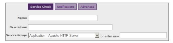
After naming and describing the check, the **Service Group** field is the most important one to look at. You can either select one that is already defined or create a new one. Note that the service group is used only within the host template's **monitors** tab for ordering and finding the checks easily.
