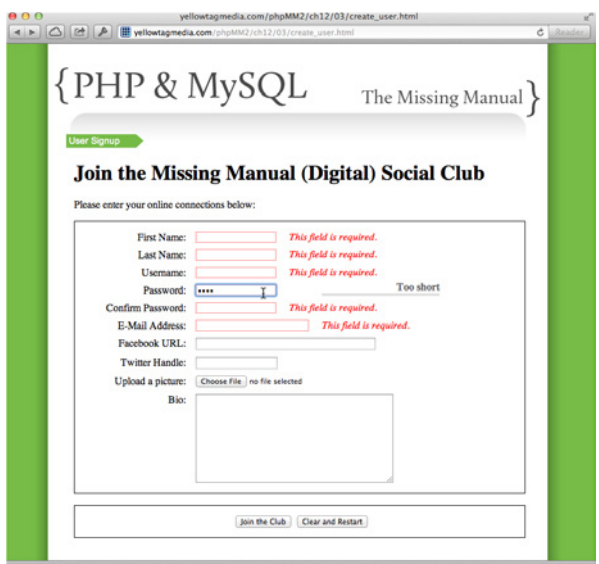
FIGURE 12-10 The password validator is an add-on for the jQuery validation plug-in. It adds a strength indicator that requires “strong” passwords. It’s a nice feature, and best of all, it doesn’t increase your work load at all. You get all this for free, before data ever makes it to your PHP scripts.
