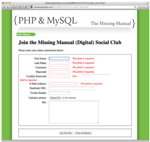
FIGURE 12-9 jQuery and the jQuery validation plug-in makes field validation a piece of cake. With minimal work, you get type validation, length validation, optionally customized error messages, and more. You can also validate emails, zip codes, and phone numbers. All that for a quick download and a few lines of JavaScript.
