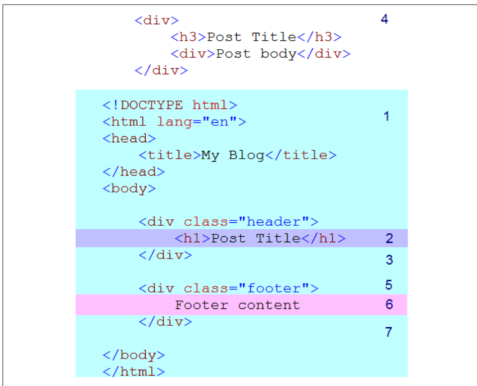
Figure 3-3. The parts of a Razor view, displayed in order of execution
