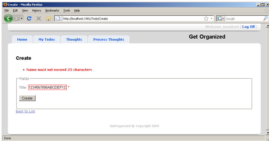
Figure 6.5: Html.ValidationSummary displays all the errors at the top of the page. Html.ValidationMessage puts an indicator next to the field that fails validation.
