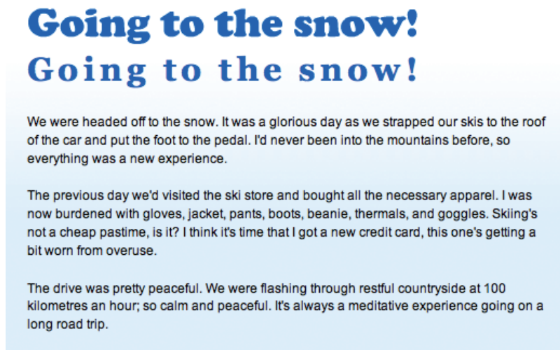
Figure 1.17: letter-spacing used to equalize metrics between Flash text and HTML text
